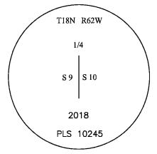
N89° 13' 06"W 5233.32' N00° 54' 56"W 2657.34' SET 3.25" ALUMINUM CAP ON 24"x5/8" REBAR N89° 31' 22"W N89° 31' 22"W 2616.35 2616.35"
